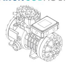
MB Frigo has developed 4 models with different cooling functions in two dimensional sizes. Condensing units are designed to work in warm climates where the air temperature can reach up to +46 ° C. Also, the evaporation working range spans from -15  $^{\circ}$  C to +5  $^{\circ}$  C.
